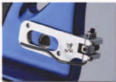
IL NUOVO REST SPIGA SLIM SOMMA LA GRANDE PRECISIONE E ROBUSTEZZA DEI NOSTRI REST Z.T. CON IL MINIMO INGOMBRO. PIASTRINA IN ALLUMINIO 1mm, BIADESIVO 3M 0,8mm, POGGIAFRECCIA SPESSORE 1,8mm.
